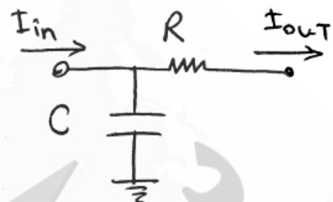
$$Z_{in} = \frac{1}{j\omega C}, Z_{out} = \frac{R}{1+j\omega RC} \quad (1)$$
