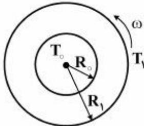
$$\frac{1}{\alpha} \frac{\partial T}{\partial t} = \frac{1}{r} \frac{\partial}{\partial r} \left( r \frac{\partial T}{\partial r} \right) + \frac{1}{r^2} \frac{\partial^2 T}{\partial \theta^2} + \frac{\partial^2 T}{\partial z^2} \quad (1)$$
