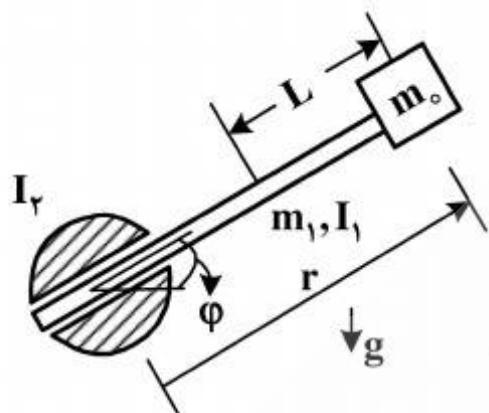
$$\frac{1}{2}I_r\dot{\phi}^2 + \frac{1}{2}I_1\dot{\phi}^2 + \frac{1}{2}m_0[r^2\dot{\phi}^2 + \dot{r}^2] + m_0g(r-L) \quad (1)$$
