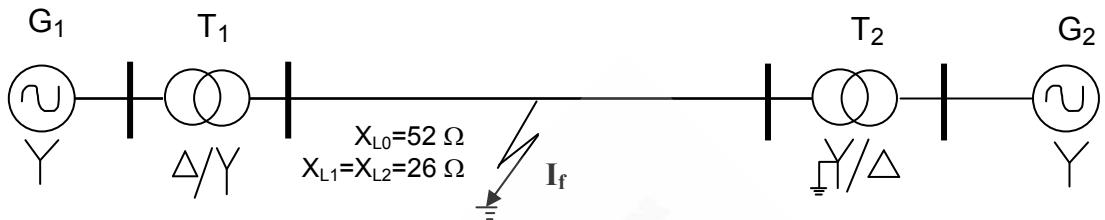
$$G_1 \text{ و } G_2 \begin{cases} 100 \text{ MVA} \\ 20 \text{ KV} \\ X_1 = X_2 = 10\% \\ X_{\circ} = 12\% \end{cases}$$
