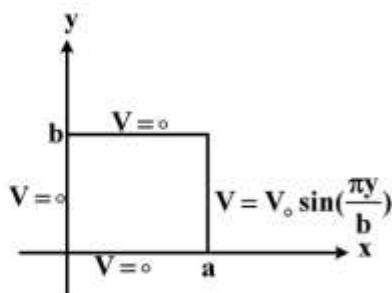
$$-\frac{\pi \epsilon_0 V_0}{b \sin\left(\frac{\pi a}{b}\right)} \sin\left(\frac{\pi x}{b}\right) \quad (1)$$
