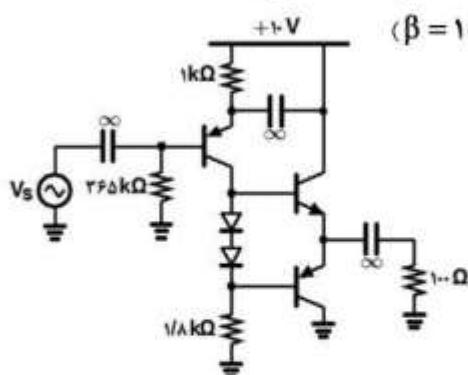
$$\text{(فرض کنید: } \beta = 100, |V_{CE,sat}| = 0 \text{ V}, |V_{BE(ON)}| = V_{D(ON)} = 0.7 \text{ V})$$
