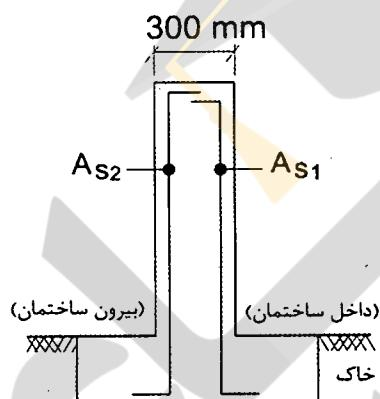
$$A_{s1}=225 \text{ mm}^2/\text{m}, A_{s2}=225 \text{ mm}^2/\text{m}$$
