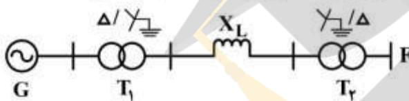
$$\begin{cases} 50 \text{ MVA} \\ 10 \text{ kV} \\ X'' = X_2 = 0.1 \text{ p.u} \\ X_0 = 0.05 \text{ p.u} \end{cases}$$
