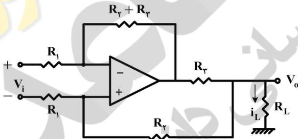
(۱)  $\frac{i_L}{v_i} = -\frac{R_2}{R_1 R_2}$
