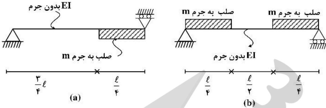
$\omega_1^a > \omega_1^b$  ,  $\omega_2^a > \omega_2^b$  (۲)
